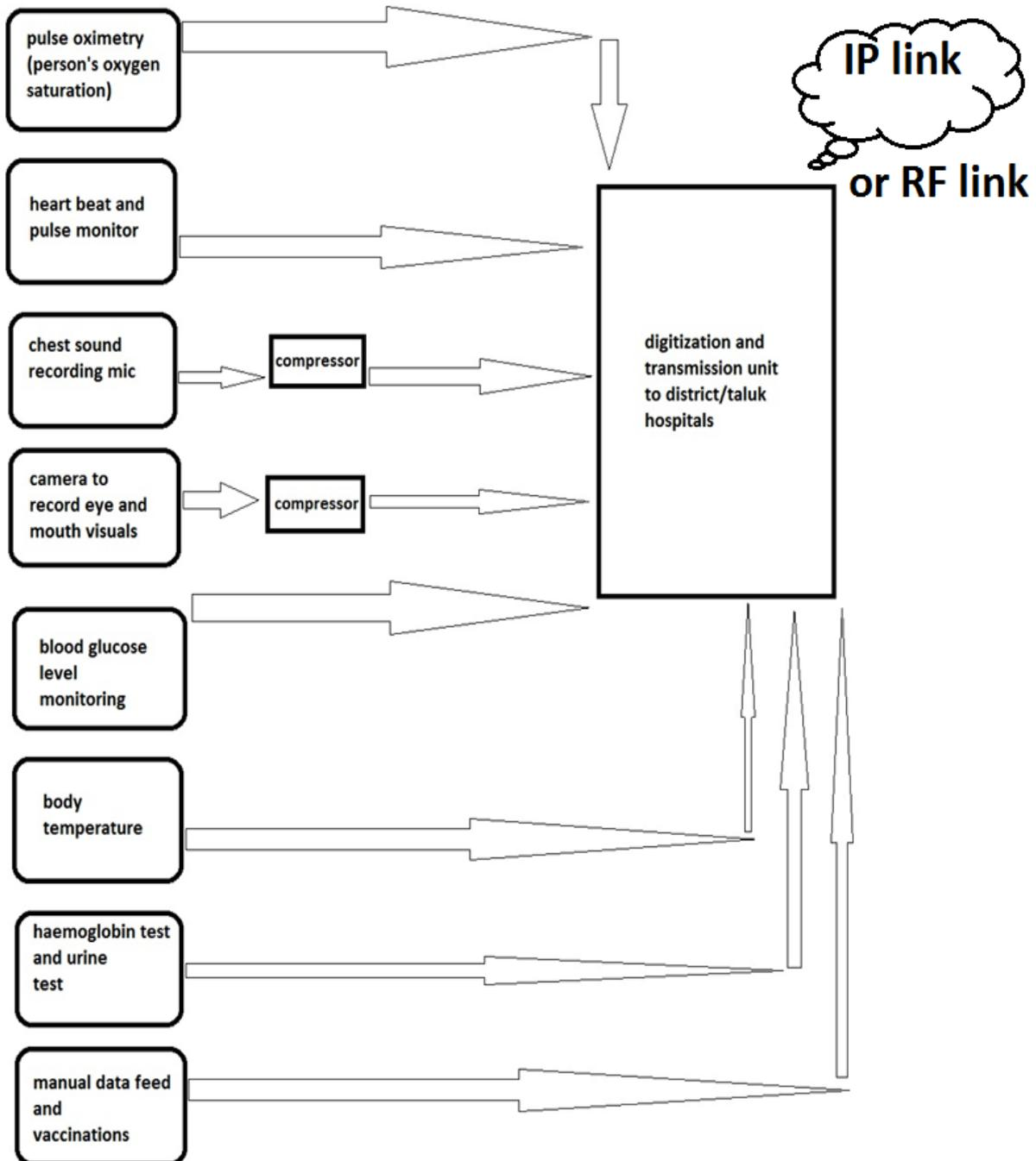
Figure 1 block diagram of the Local clinic unit/Anganwadi unit
